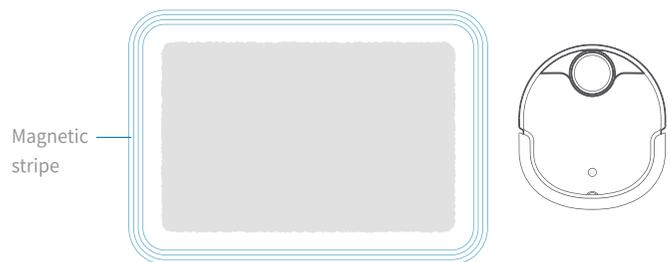
5. It is recommended that the robot be used in two-storey rooms with a fence or magnetic strip presence. ⚠️
