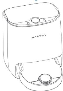
**12.** After completing a mopping task, the robot will return to the base station to get the mop cleaned and air dried automatically.
