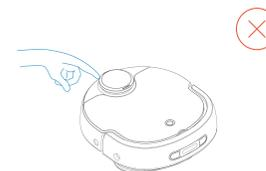
**3.**To avoid injury, keep hair, fingers, or other parts of the body away from the mop, side brush, LIDAR, vacuum port, or cleaning board of the robot.
